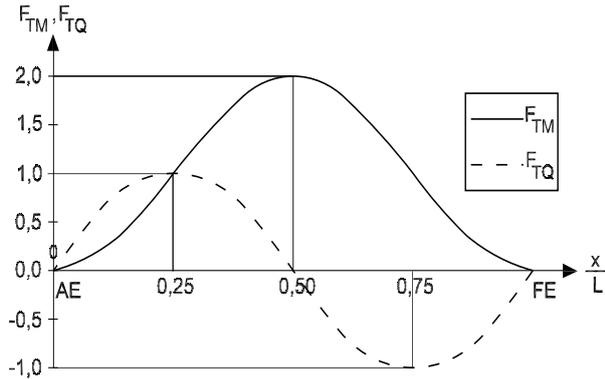
**Figure 6 : Unit condition 2 - Distribution factors  $F_{TM}$  and  $F_{TQ}$**
