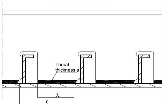
**Figure 5 : Intermittent scallop fillet welding between cut-outs**
