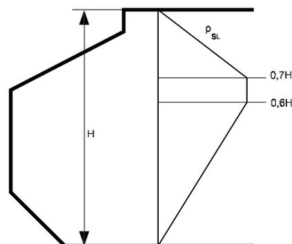
**Table 4 : Reference pressure for calculation of sloshing pressures**
