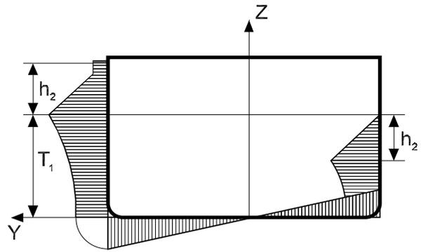
Figure 5 : Wave pressure in load case “d”
