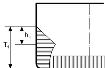
Figure 3 : Wave pressure in load case “b”
