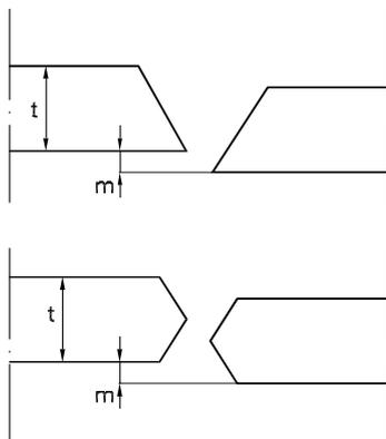
Figure 13 : Misalignment in cruciform connections
