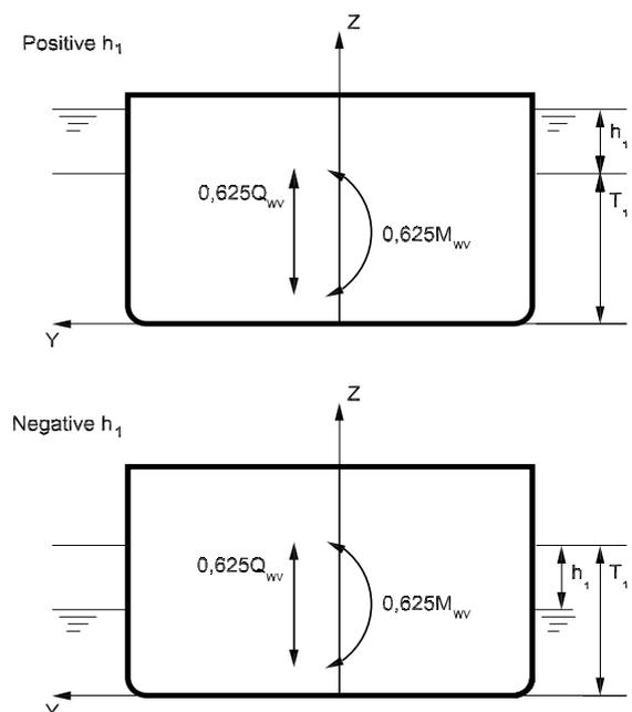
Figure 2 : Wave loads in load case “b”
