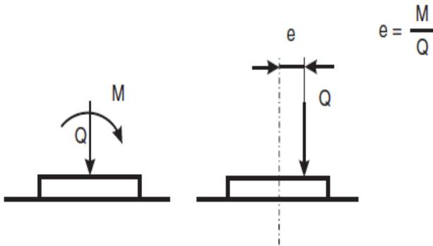
For rectangular base area of length  $L$ , in m, and width  $B$ , in m, and load eccentricity  $e$ , having components  $e_1$  and  $e_2$  along the length and width, respectively, the following results (see Fig 2):
