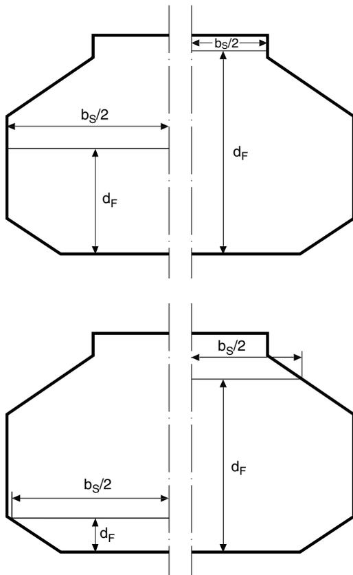
**Figure 5 : Breadth  $b_s$  of the free surface of the liquid, for units with longitudinal bulkheads**
