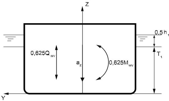
Figure 3 : Wave loads in load case “c”
