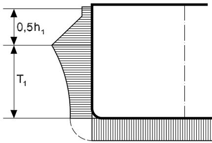
Figure 4 : Wave pressure in load case “c”
